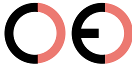
False CE Mark (too far)
